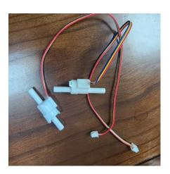
The water flow sensor mainly consists of a copper valve body, a water flow rotor component, and a Hall sensor.
